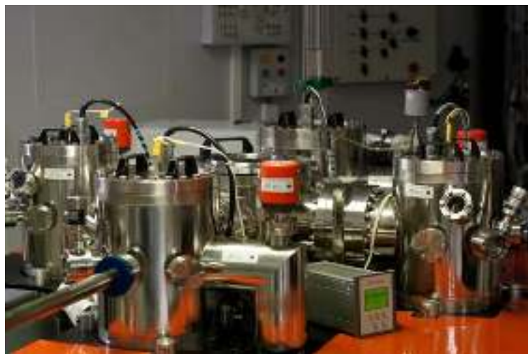
Figure 2.15 ELECTTRORAVA PECVD system existent in CEMOP used for the deposition of the Silicon thin layers.
