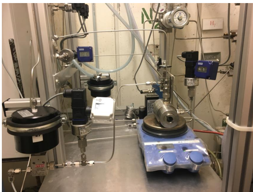
Figure 4. Experimental apparatus used for the continuous mode of the coupling reactions between limonene oxide and CO 2 .
