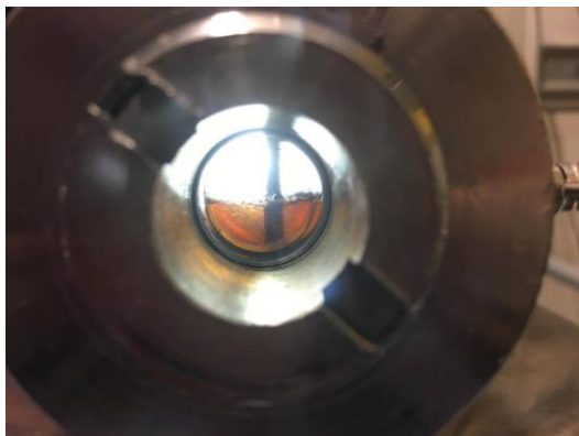
Figure 3. Detail of the deep tube inside the high pressure reactor used for the continuous mode reactions.
