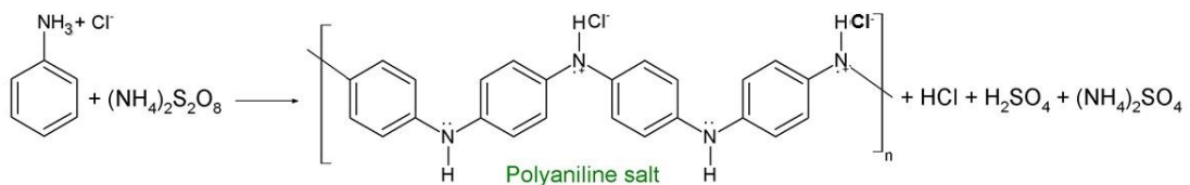
Figure 3.1 - Chemical oxidative polymerization of aniline monomer by ammonium persulfate.
