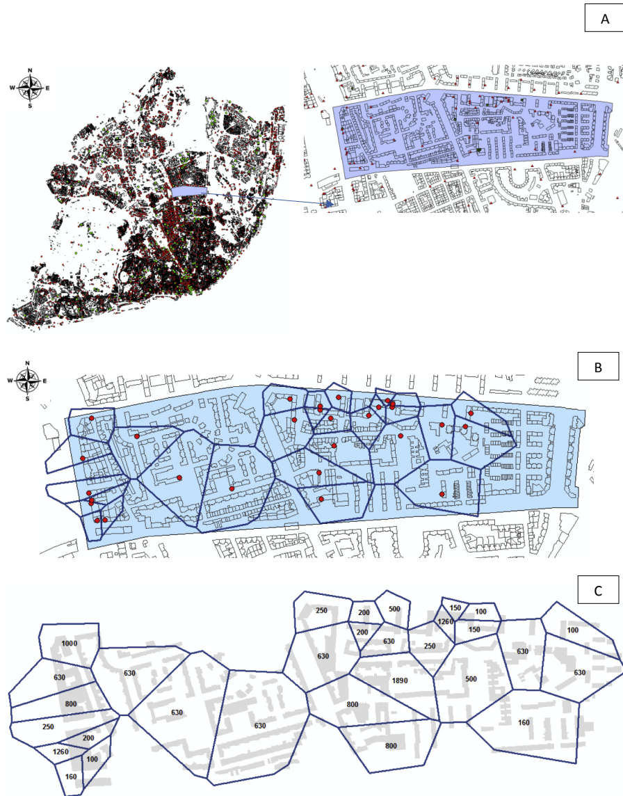
Fig. 1. Delimitation of Alvalade (blue area) and location of the transformers (red dots) (A), Thiessen polygons depicting the influence zones of all transformers (B) and transformer power capacities [kVA] (C). (For interpretation of the references to colour in this figure, the reader is referred to the web version of this paper.)
