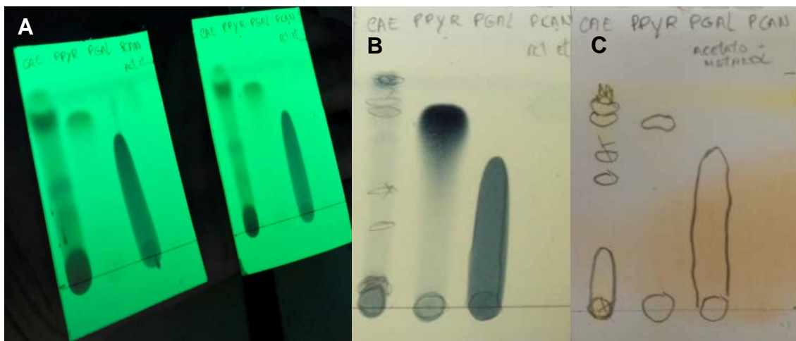
Figure 33 (A) Carqueja extract obtained with ethanol, observed under UV light. (B) Same Carqueja extract after spraying with the universal stains phosphomolybdic acid and (C) 3,4-dinitrophenylhydrazine.
