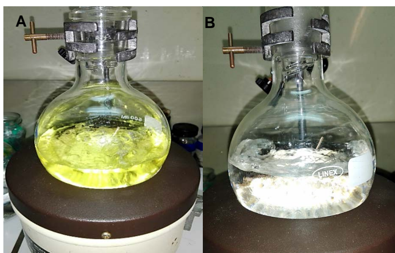
Figure 28 Images of Soxhlet extraction of Carqueja with n -hexane (A) at the beginning and (B) end of the assay.
