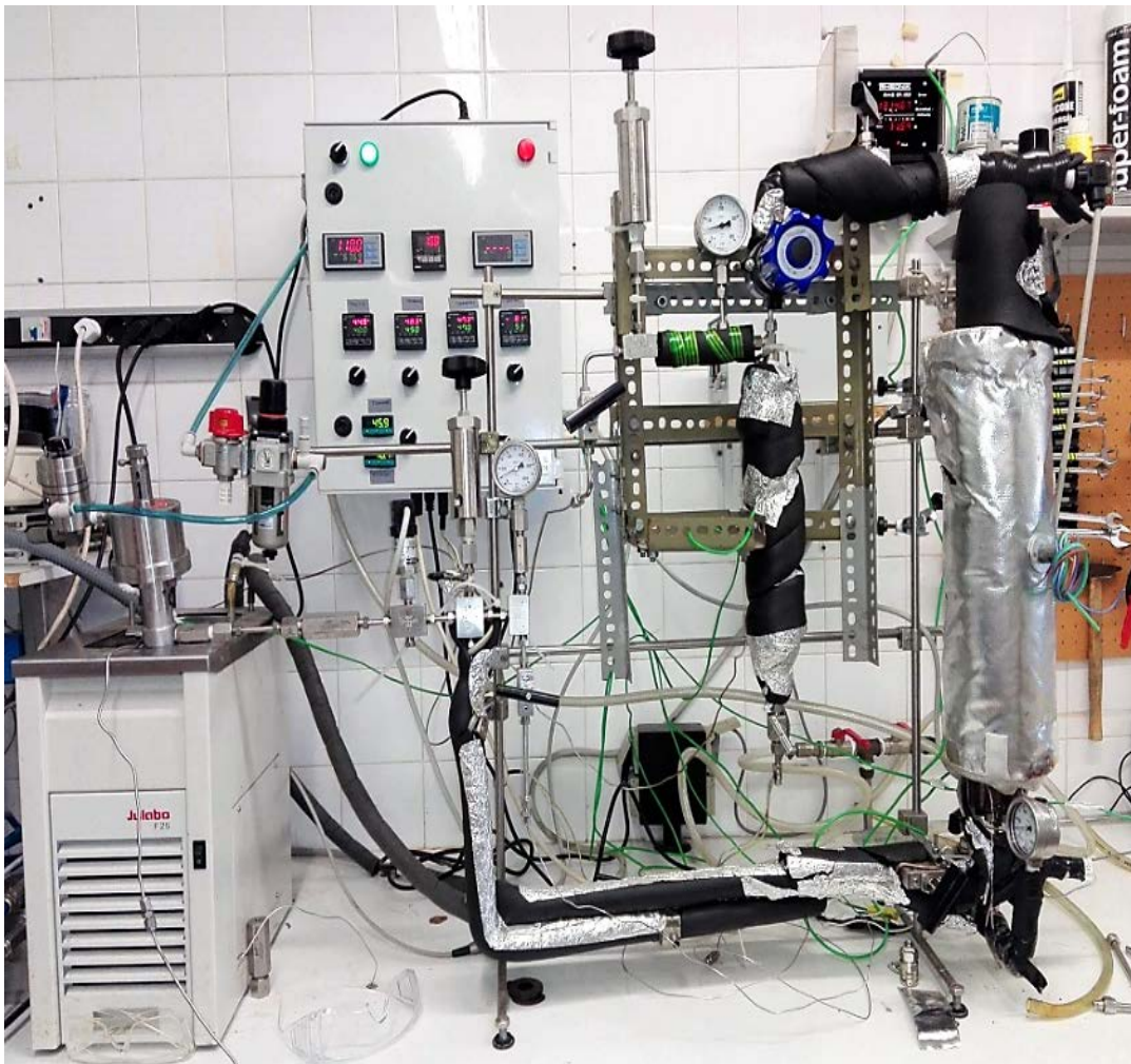
Figure 16 Image of the scCO 2 extraction apparatus.
