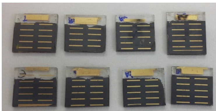
Figure 47: Solar cells batch of perovskite films deposited over compact and mesoporous \text{TiO}_2 ETL using 1 M and 1.5 M solutions concentration.
