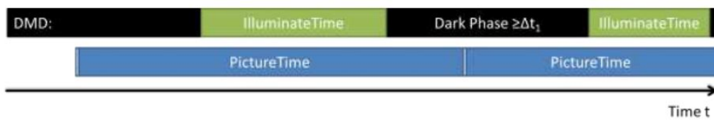
FIGURE A.1: Vialux DLP V-7000’s timing settings [77].
