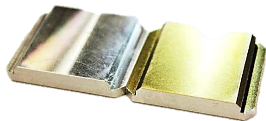
(b) pull-out tab before (left) and after (right) laser treatment
