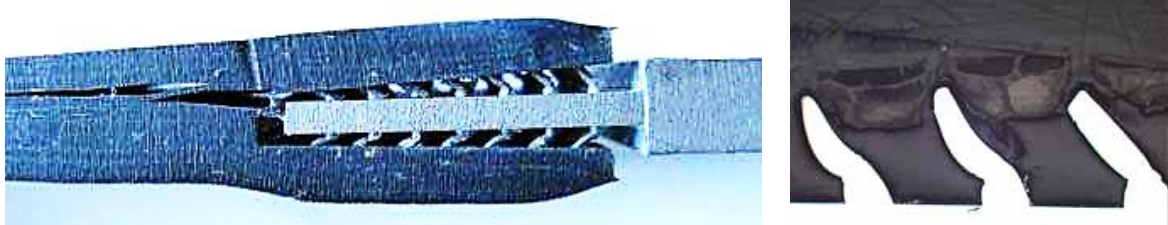
Fig. 9- CMT-reinforced (cylinder pins) double-lap failed shear joint [26].
