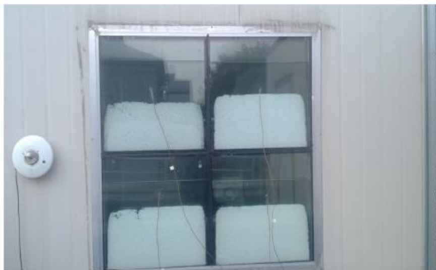
Fig. 4.33. The melting state of the PCM in the rainy summer day (14:00) [152]
