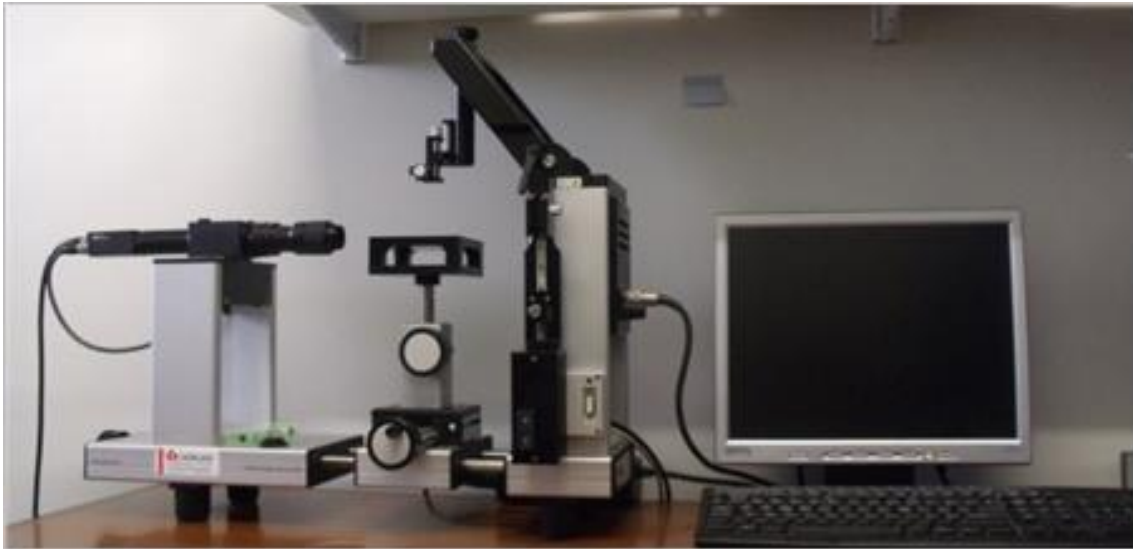
Figure 3.2. Apparatus model OCA 15 Plus (Dataphysics Instruments, Germany), for contact angle measurements after capturing of the drop image in the surface of bacterial lawns with a video camera.
