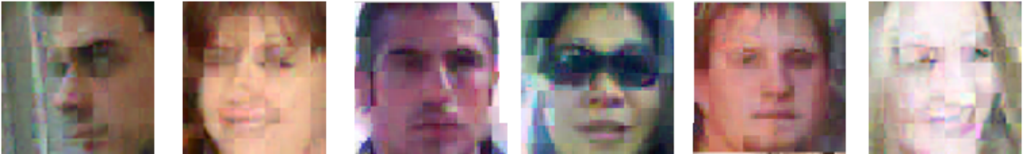
Figure 4.12: Patch-based reconstruction We verify that 6 \times 6 pixel patches are sufficient by reconstructing the original images using the closest patches l^* from the library. It is still easy to identify the pose of the images using the approximated versions. Note: for illustration purposes the RGB form of the test and library images were used in this case to produce the reconstructed images above.
