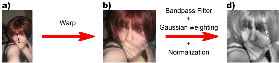
Figure 3.6: Face preprocessing: (a) We manually place 2 landmarks on the face at the bridge of the nose and the top of the mouth. (b) We then warp the images to a 60x60 template using a Euclidean transformation. (c) We then band-pass filter the images using lower and upper cutoff frequencies of 2.5 and 25 cycles per image respectively and weight the pixels using a Gaussian function centered on the image. Finally, each image is normalized to have zero mean and unit standard deviation.
