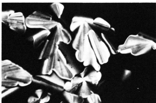
Fig. 4. A photographic picture of the texture of the mesophase of 4f taken at 124 °C using a polarizing microscope (Magnification \times 160 ).
