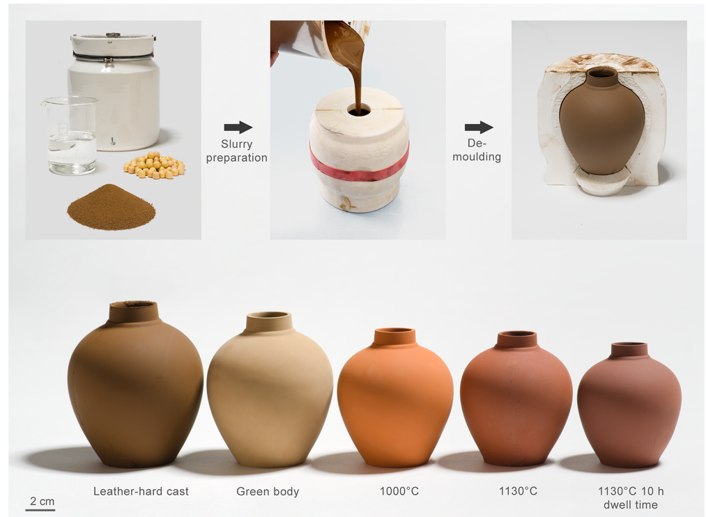
Fig 4. Vases slip cast with the JSC-Mars-1A slurries. Top panel: Slip casting fabrication procedure of vases. Bottom panel: Vases, from left to right: directly after demolding, dried green body, 1000 °C without dwell time, 1130 °C without dwell time, 1130 °C with 10 hours dwell time.
