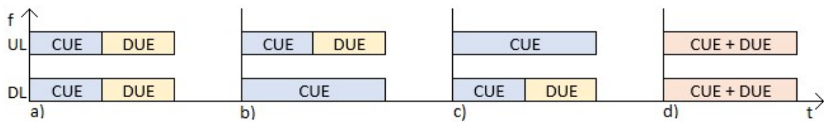
Figure 2.1: a) Cellular mode, b) Dedicated mode (uplink), c) Dedicated mode (downlink), d) Shared mode
