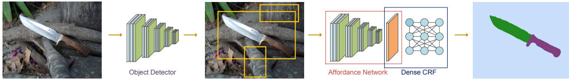
Fig. 3.4. An overview of our Sequential Architecture. From left to right: A deep network is first used as an object detector to generate the object bounding boxes that narrow down the region of interest. A second network is then used to produce feature maps from these bounding boxes. Finally, these maps are post-processed with dense CRF to improve the prediction along the class boundaries.
