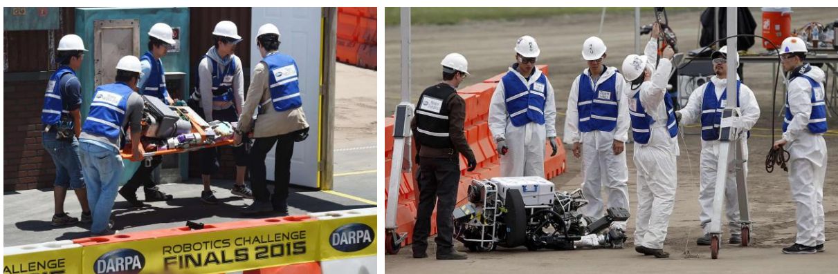
Figure 1-3: Pictures show the devastating effect of humanoid fall overs and as a result humans had to intervene to carry them away.
