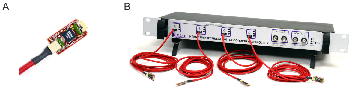
Figure 3.2.2: INTAN setup used in the Injured Anesthetized experiments. A) RHS2116 16-channel stimulation/recording headstage. B) Intan RHS2000 Stimulation/Recording Controller front panel.
