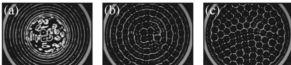
FIG. 13. Series of snapshots of the principal pattern evolution of the magnetic fluid for a jump from B_0 < B_c to B > B_c , illuminated from above by a ring of LEDs. The pictures are taken \Delta t = 180 ms (a), 280 ms (b), 560 ms (c) after the start of the increase of the magnetic field.
