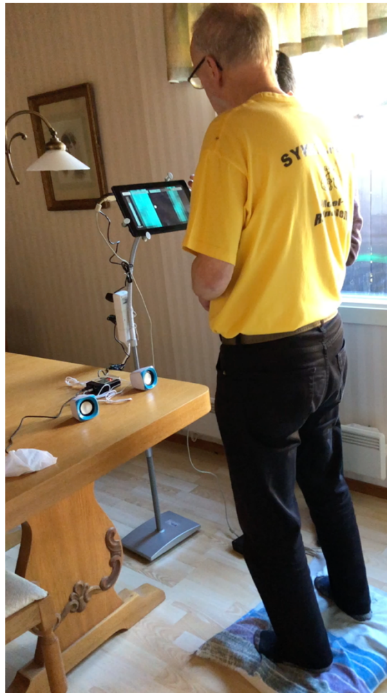
Figure 2. The balance foam, together with the feedback devices – a tablet for the visual presentation, and loudspeakers for sounds.
