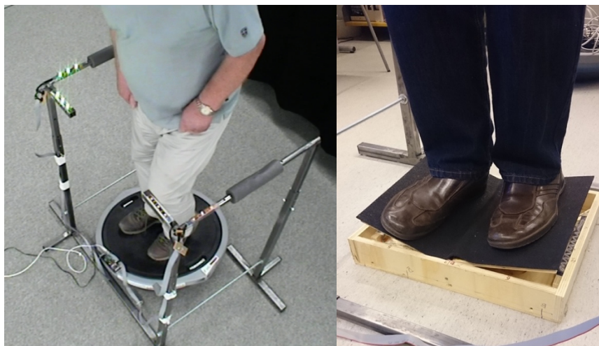
Figure 1. Left: Stroke survivor using the interactive bosu ball, leaning slightly to the right. Therefore the right hand lights are lit up. Right: The pedals. These pedals are linked together with a rubber sheet, and the same safety handle bars as in figure 1 were used.
