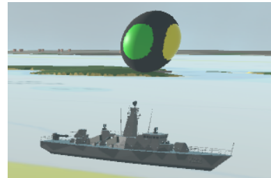
Figure 10: From the AIS data, the ship type, position and heading is extracted. From the ship type, a suitable 3D-model is chosen. The sphere is positioned above the position, and is colored according to the heading.
