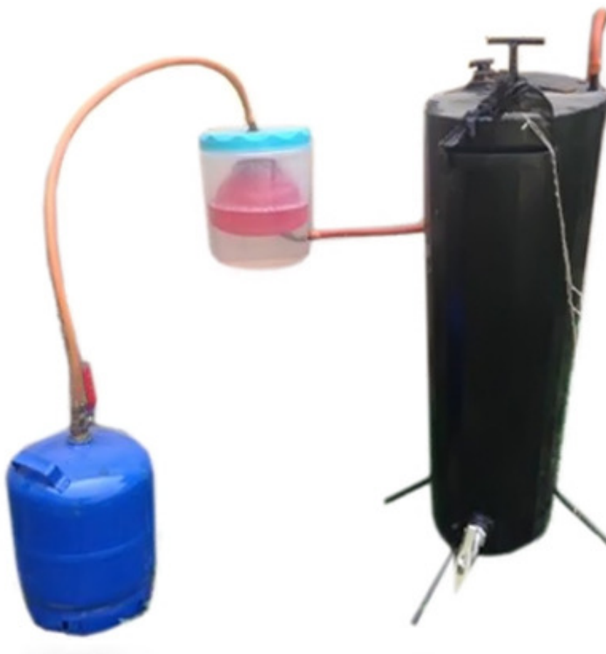
Plate 1 Experimental setup of the anaerobic digester
