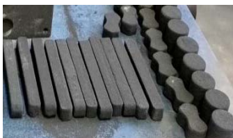
Figure 5: Transverse bars and tensile specimens.
