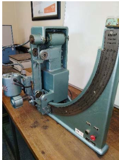
Figure 3: Ridsdale and Dietert Universal machine
