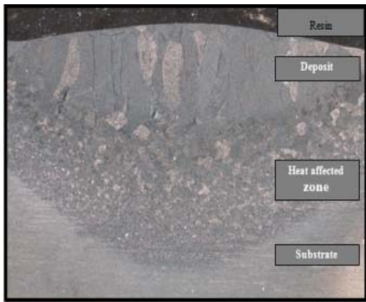
Fig. 4. The microstructure of sample at a laser power of 1.2 kW showing the deposit zone, and heat affected zone.
