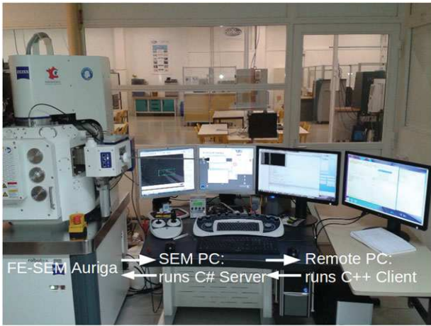
Fig. 1. The setup with the Zeiss Auriga FE-SEM and the associated PC.
