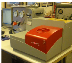
HP μ-DSC (SETARAM DSC-7) P < 400 bar ; -45 °C < T < 120 °C
