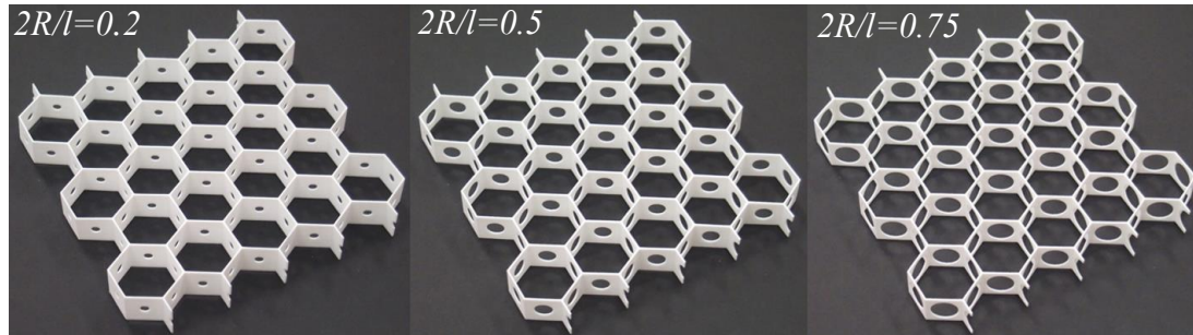
Fig. 4.22. 3D Printed perforated honeycomb specimens with 2R/l=0.25 , 2R/l=0.5 and 2R/l=0.75 , from left to right.
