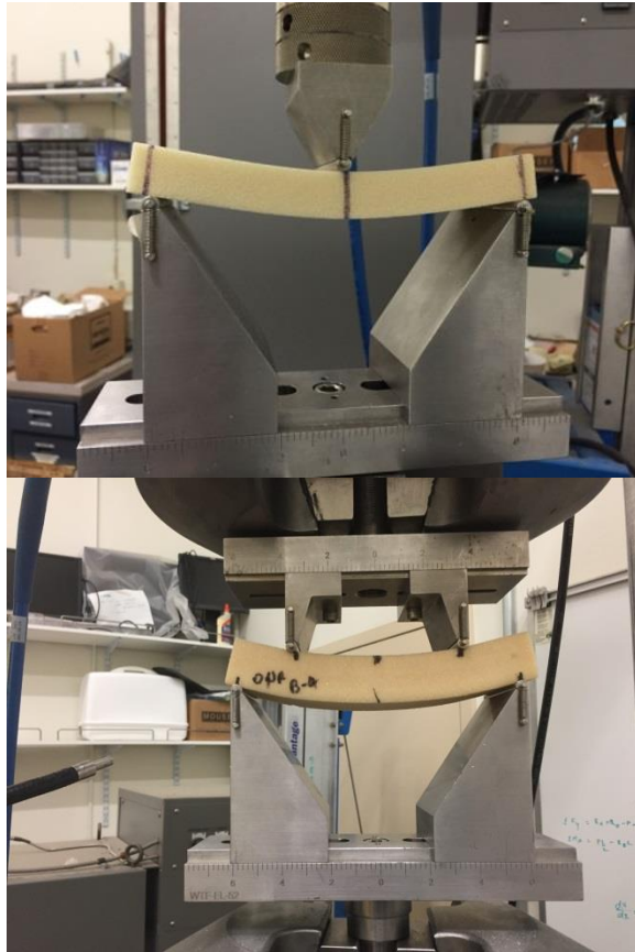
Figure 4-1 : Three and four point bending tests
