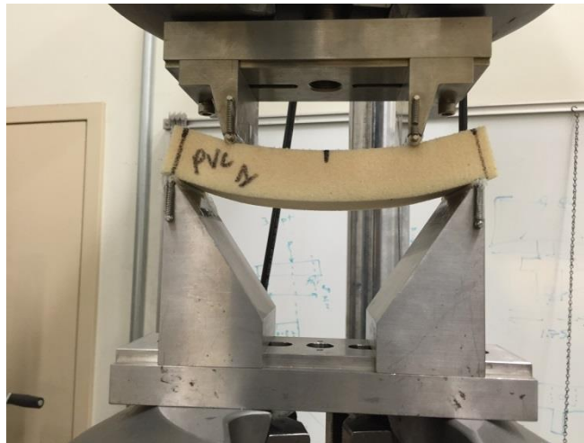
Figure 5-31: Four point bending test on PVC foam
