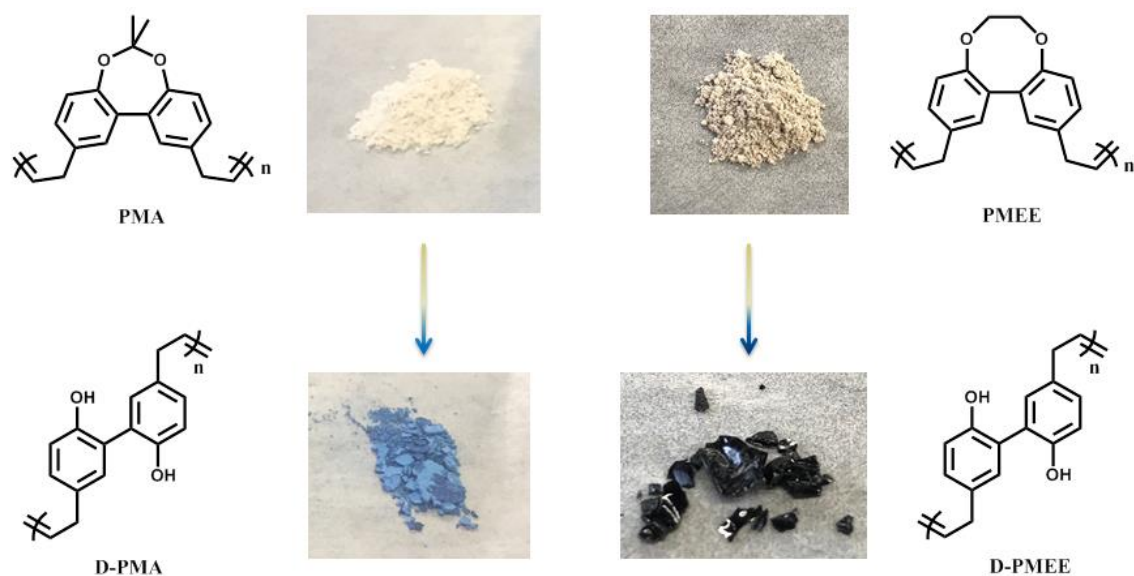
Figure 4-5. Deprotected Polymer Showing Distinct Color Change Potentially Resulting from Increased Conjugation in the Polymer Backbone. Structures are Idealized Repeat Units Resulting from No Isomerization.
