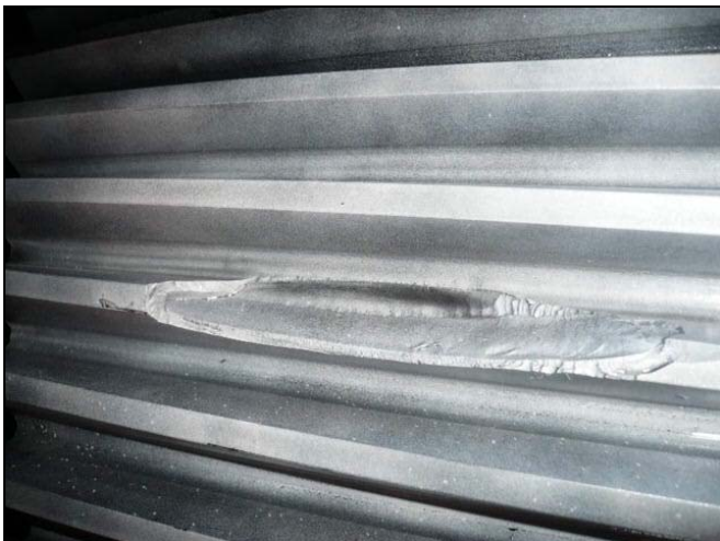
Figure 31. Gear Tooth Breakage.
