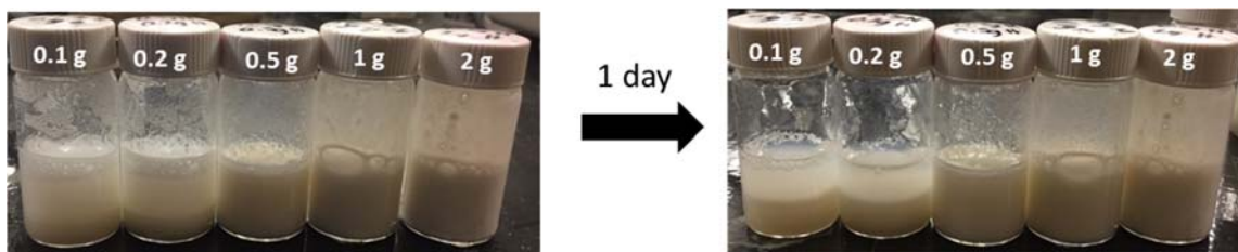
Figure A. 40 Colloidal Dispersion of HNT in Water in Aid of Hydroxyethylcellulose. Digital photographs of colloidal dispersions of HNTs dispersed in 10 mL water with the help of 0.5 g of hydroxylethylcellulose. The digital photographs in the left panel were taken immediately after mixing, whereas the panel on the right was photographed 24 h after mixing.
