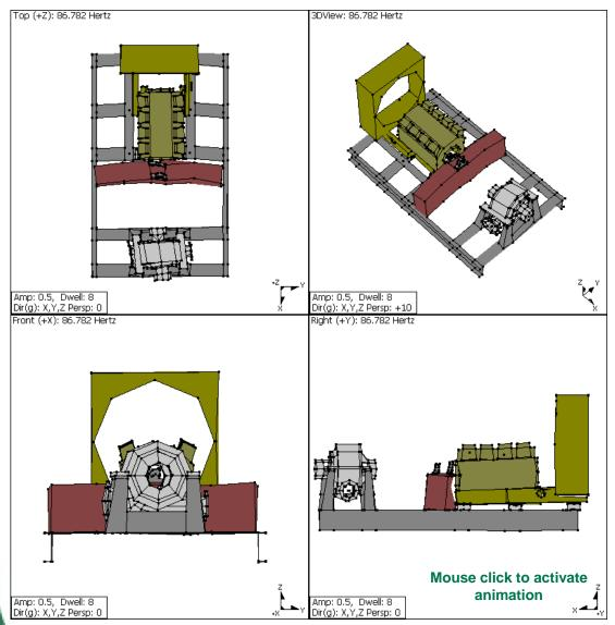
3x rpm (86.8Hz or 5,208 rpm)
