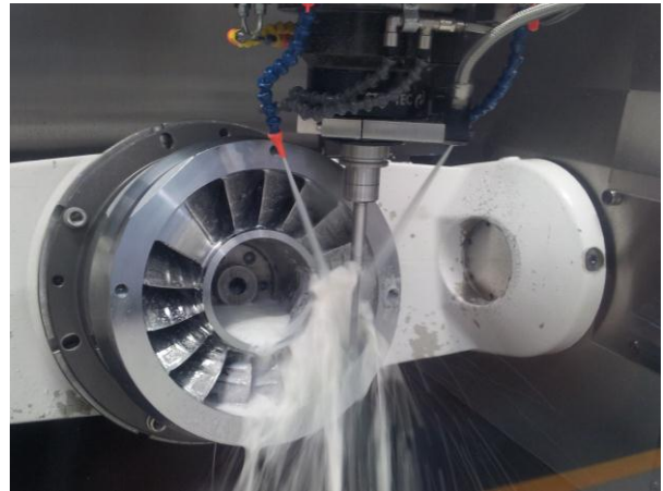
Figure 11 IN718 impeller under rough turning operation
