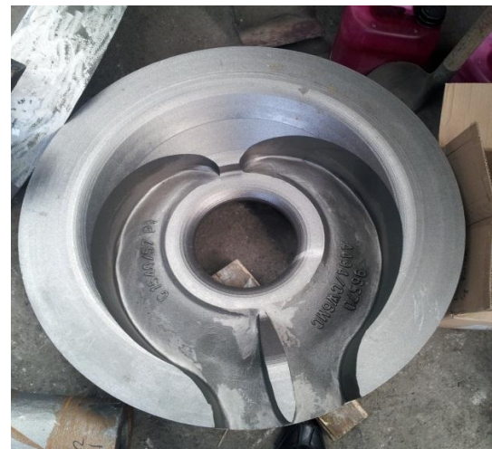
Figure 12 Casted Diaphragm in IN625
