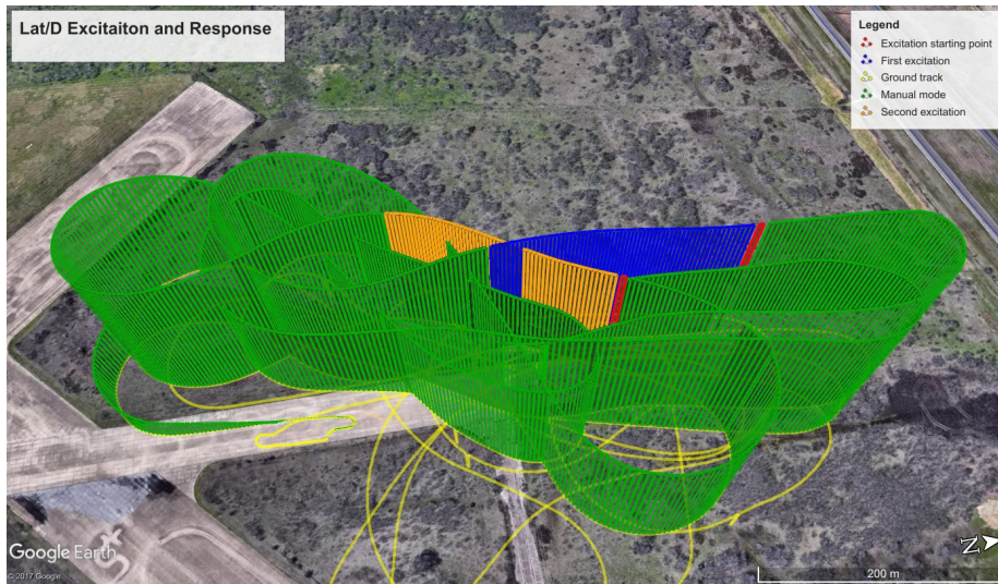
Figure 6.6: Flight path of a lateral/directional path using the developed automated excitation method.
