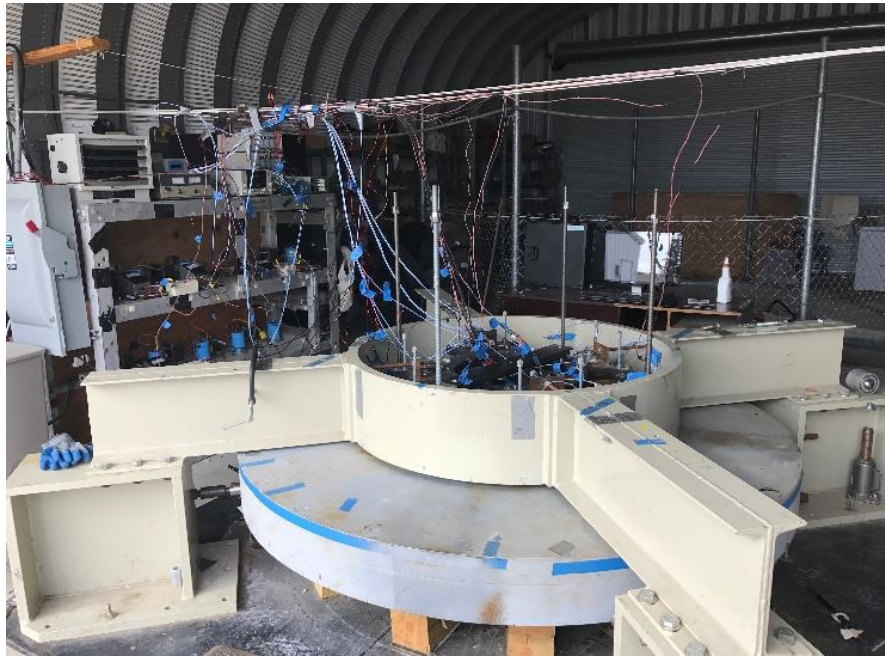
Fig. 53 The Texas A&M shaft-less flywheel-CAMB assembly.
