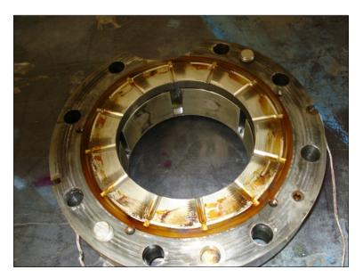
9. On both bearings, journal pads and thrust faces were showing signs of high temperature exposure.
