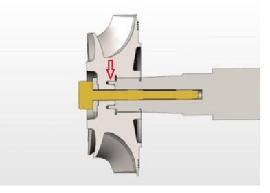
New machining design applied to the shaft and wheel.
