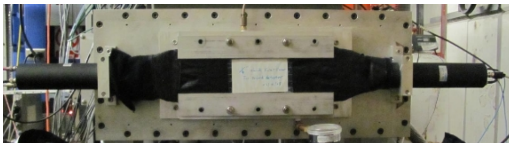
Figure 3.8: Photograph showing the back of the Oxford detector with the scintillator and 2 phototubes.
