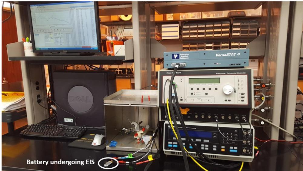
Figure A-3: Battery undergoing EIS
