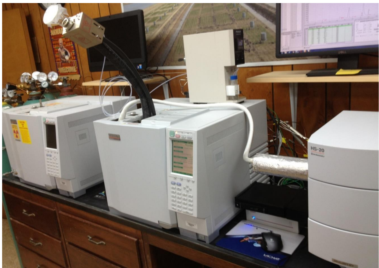
Figure 2.3. The Gas Chromatography-Mass Spectrometry (GC-MS) set-up used for estimating 2-Acetyl-1-pyrroline (2AP).
