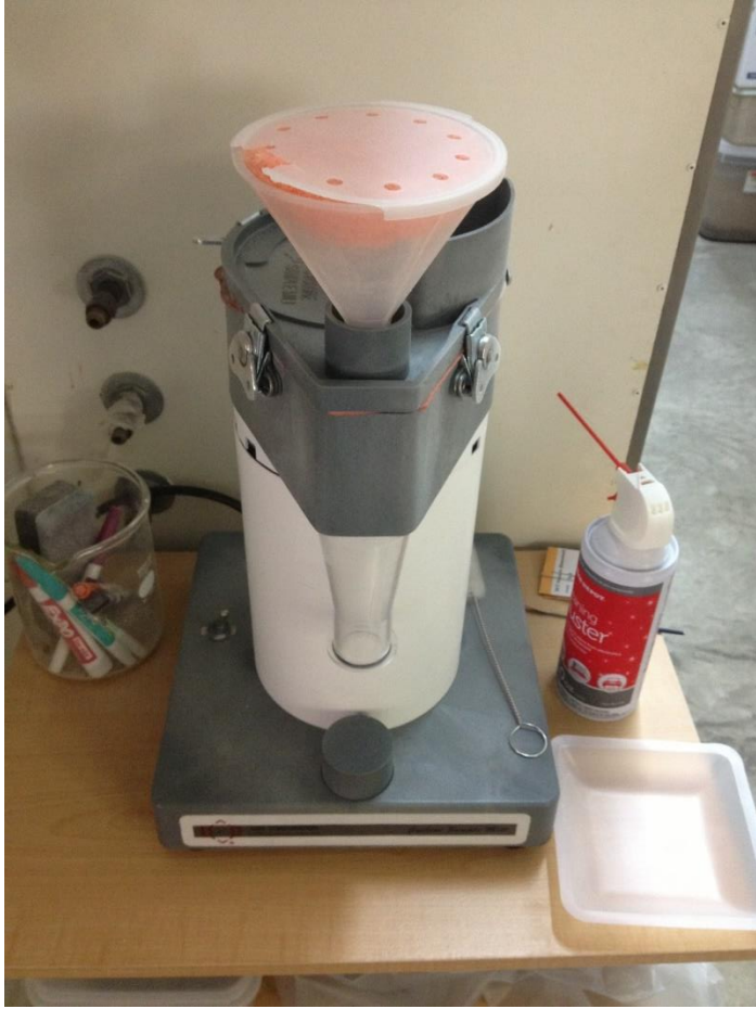
Figure 2.2. Cyclone lab sample mill used for grinding milled rice.
