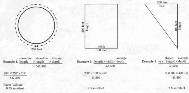
Figure 2. Determining Pond Water Volume
