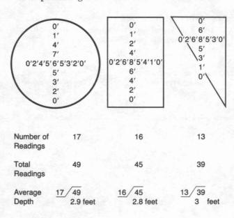
Figure 1. Determining Average Depth of Ponds
