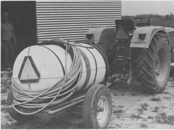
Fig. 2. Washing and disinfecting equipment must be capable of delivering 200 to 400 lbs. of pressure.
