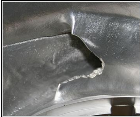
Figure 2: G-2001 old rotor 2 nd stage vane inlet
