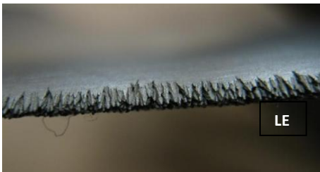
Figure 17. Compressor blade exposed to WDE process.
