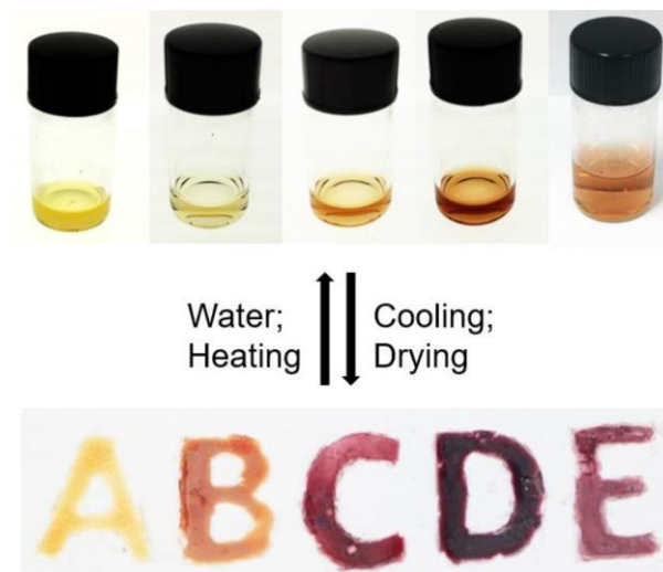
Figure 3.20 Photographs demonstrating the recyclability of the thermochromic materials based on 1\cdot4\text{Br}\rightarrow 2\mathbf{a}-2\mathbf{e} . These materials can be easily recycled by dissolving in hot water. The regenerated aqueous solutions can be used to prepare new thermochromic patterns.
