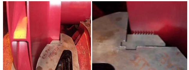
Figure 9. Polymer eye seals installed in DuPont's charge gas compressor.
