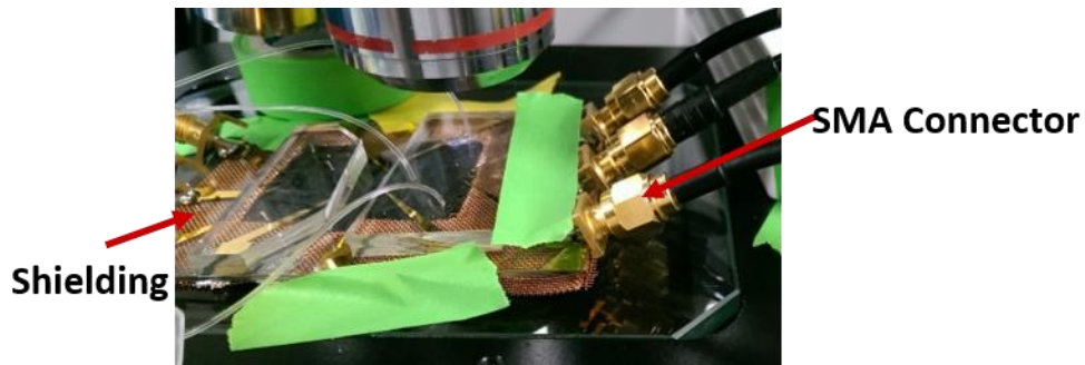
Figure 23. The fabricated microfluidic impedance spectroscopy platform integrated with SMA connectors.
