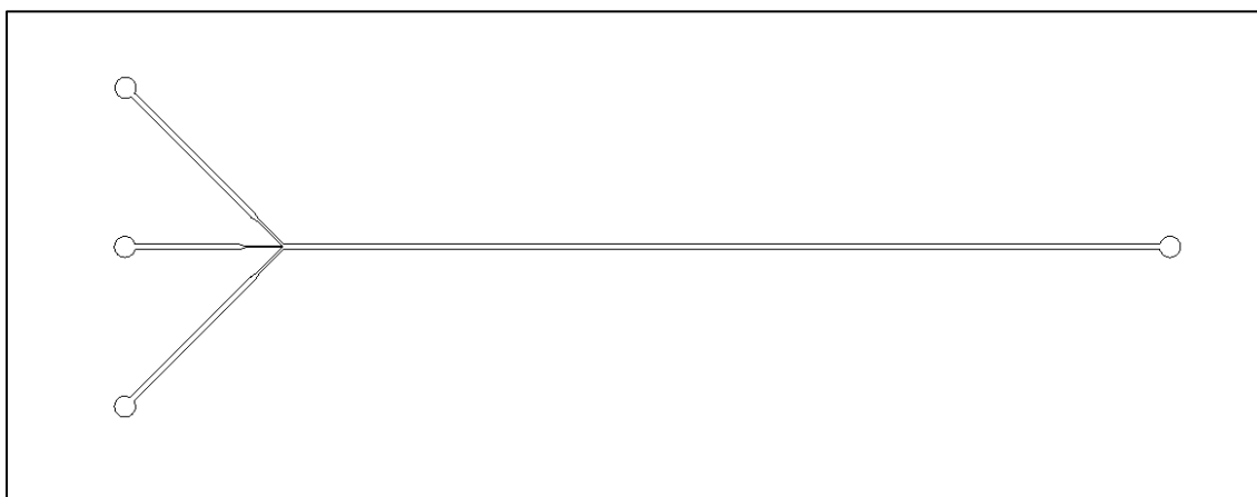
Figure A. 1: Cell and particle position detection microfluidic channel. (File name: Particle position detection-microfluidic channel.dwg).
