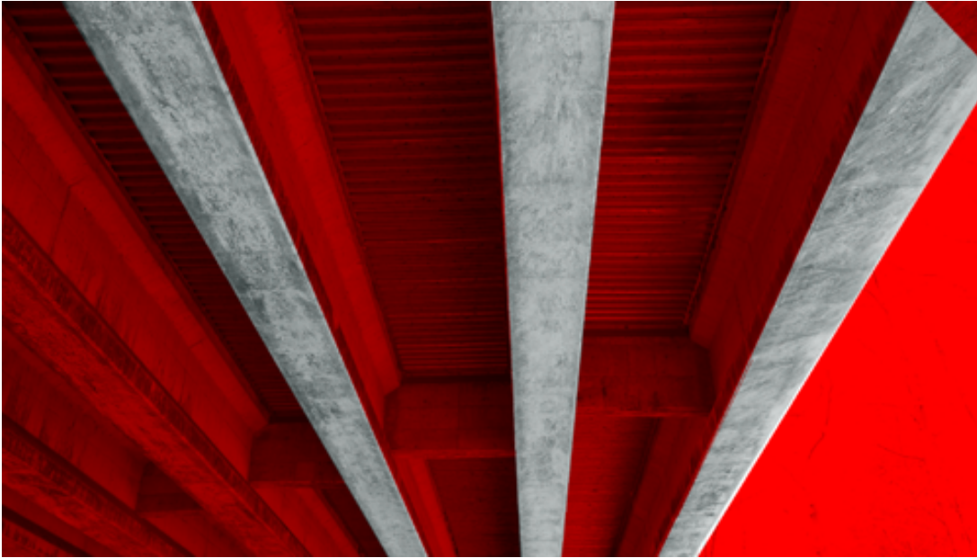
Figure 6.3. The original image containing only the beam flange (gray) projected onto the subsequent image (red).
