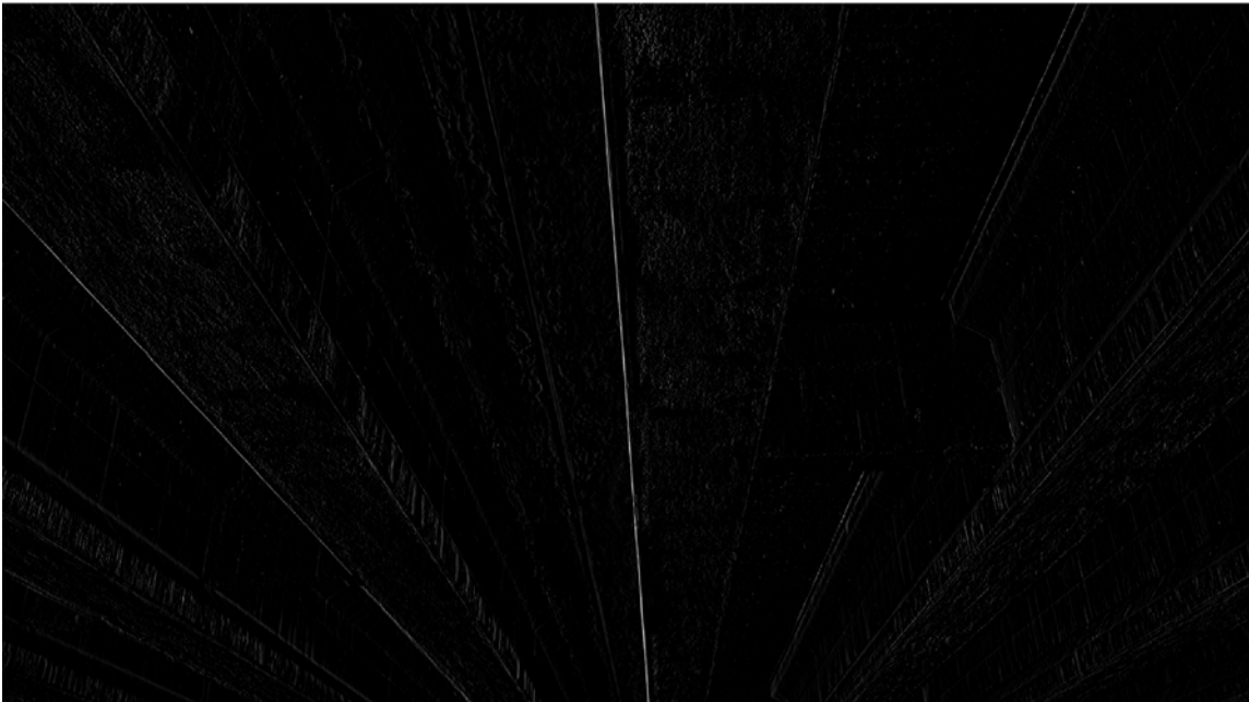
Figure 3.3. The smoothed gradient of the original image in the horizontal direction.
