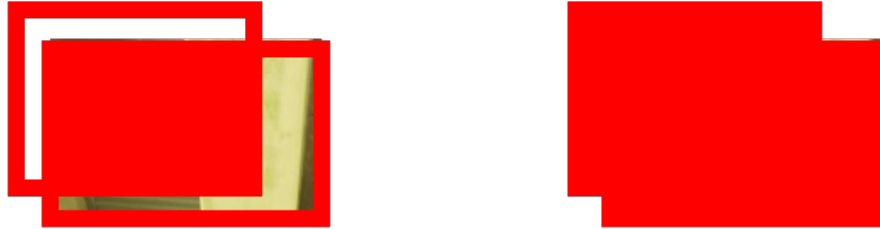
Figure 3.13. An example of determining the intersection (left) and union (right) for a ground truth and a candidate.
