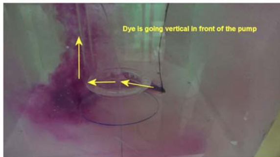
Photo 5-2 Stalling and Lifting in Front of Pump - Flow Should Towards Pump
