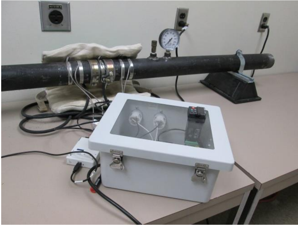
Figure 16. The physical test setup used in experimental work. Pipe heaters and thermocouples are attached to the compressed air line with an insulation blanket wrapped around the outside.
