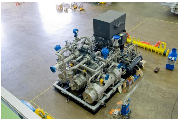
Figure 2. Integrally Geared Fuel Gas Compressor Sitting Atop Three Inter-Coolers with Motor in Background.
